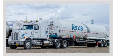
A tandem or tridem tractor and tridem trailer configuration is proposed for the transportation of LNG from the Energy Centre to customers. This configuration brings with it key advantages:
