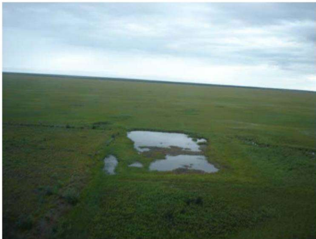
Photograph 1. Example of sump cap subsidence and surface water ponding over half of the sump area, Kugpik L-46 sump. Taken July 2013.
