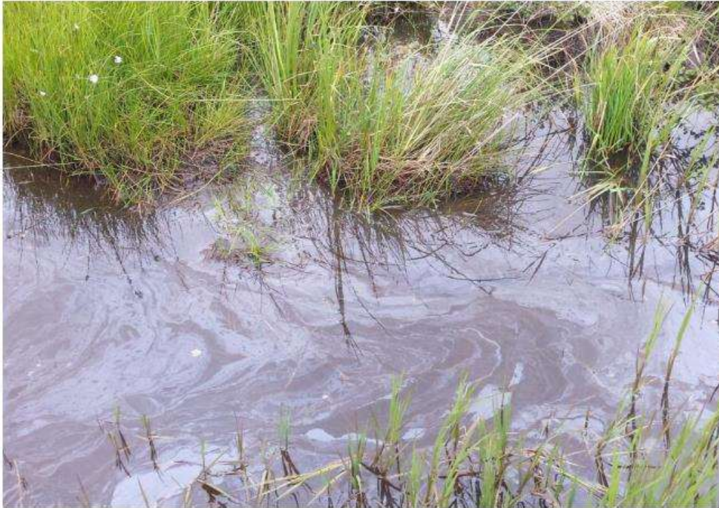
Photograph 8. Example of hydrocarbon sheen on surface water indicating potential leaching from sump, Umiak N-05 sump. Taken August 2016.
