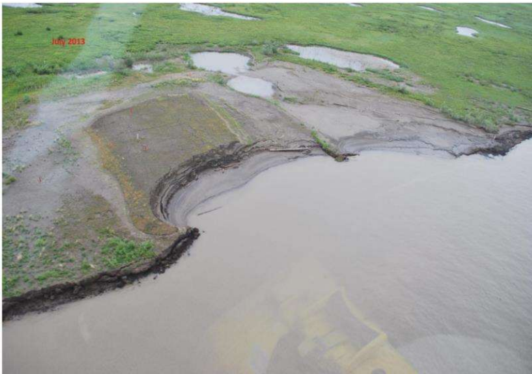
Photograph 5. Example of shoreline erosion of sump area, Unipkat I-22 sump. Sump was previously excavated of all drilling waste and backfilled with clean material. Taken July 2013.
