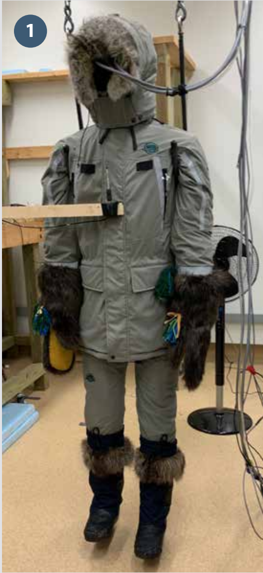
1 NEMO, the NRC thermal manikin in our St. John's laboratory, with the Parks Canada uniform and some of the Indigenous-made clothing being tested.
